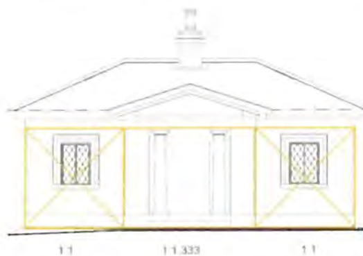
Fig. 13 Front façade – Proportion analysis – Outer bays of facade below entablature in proportion of 1:1. Central bay 1:1.33
